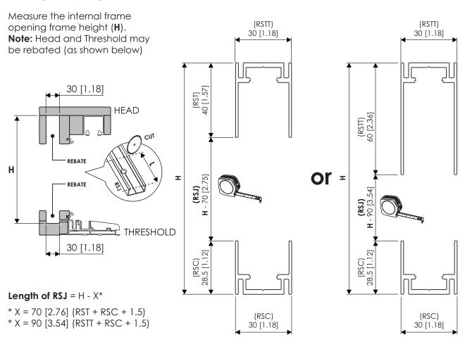
Note: For Double Screen Install, 2 RSJ Extrusions are to be cut and installed
