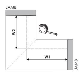
Length of RSC (W2) / RST or RSTT (W2) = W2 and Length of RSC (W1) / RST or RSTT (W1) = W1
