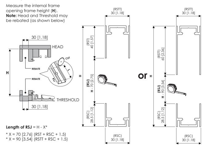
Note: For Corner Double Screen Install, 2 RSJ Extrusions are to be cut and installed
